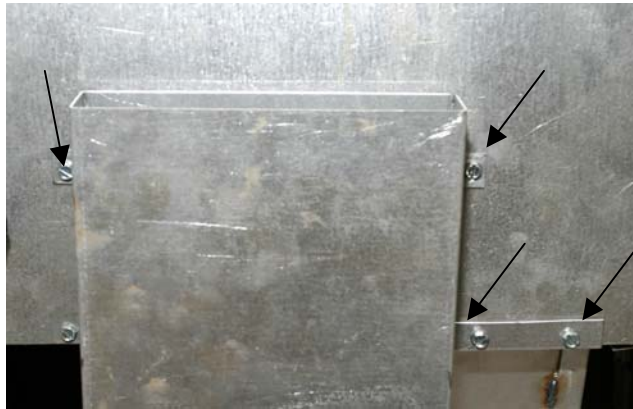
Figure 2: The screws, which secure the blower and flue assembly to the back of the fryer, are marked with arrows.
