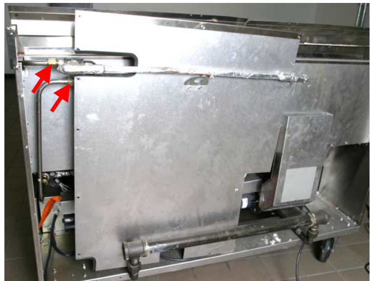
Figure 1: Removing a one-piece back requires disconnecting the oil return lines at the arrows. The gas manifold should also be removed.
