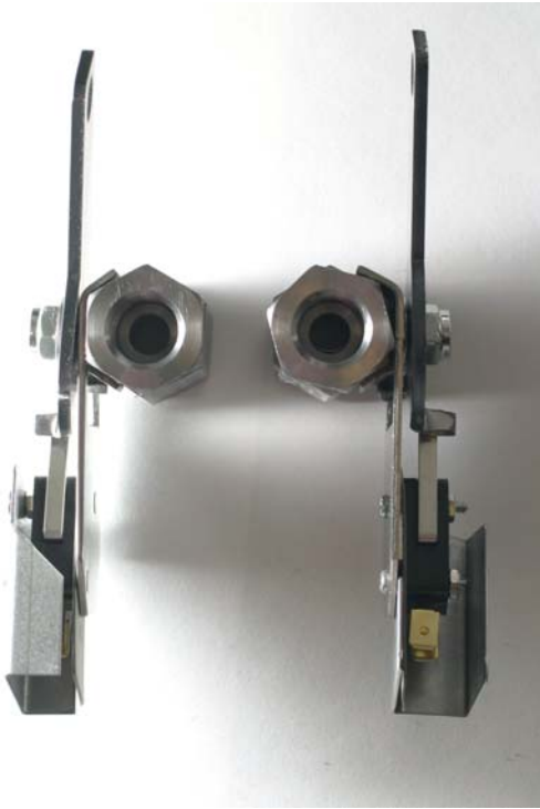
Figure 8: Flush valve actuators and microswitches are shown for left and right-hand mounting. The parts are not interchangeable. The flush handle should be pulled forward to open the drain and activate the pump.
