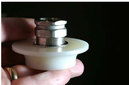
Figure 12: The new quick-disconnect is cut away to allow easier handling and to take advantage of the emboss in the filter pan lid.
