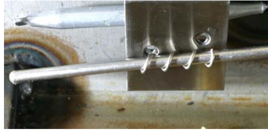
Figure 15: Position the provided spring over the temperature probe shaft as shown above.
