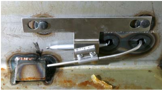
Figure 16: On units without a probe bracket, position the provided bracket on the frypot studs and secure the temperature probe as shown. The hi-limit can rest behind the bracket.
