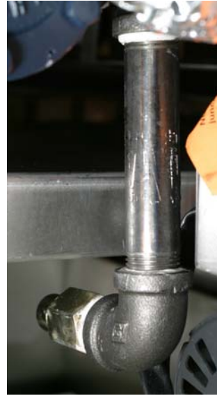
Figure 11: The new, shorter oil return nipple and elbow are shown in place. The nipple must face straight forward, ensuring the filter hose curves away from the blower housing when the filter pan is in place under the fryer.
