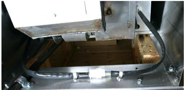
Figure 3: The routing for a blower harness on a new unit is shown. Units with less than two P-clamps should have an additional clamp added and the longer extension added.
