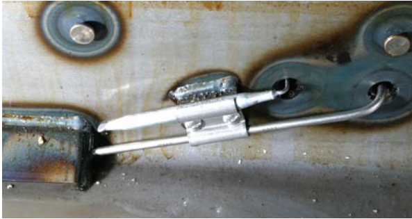
Figure 14: The hi-limit and temperature probe are attached with a bracket to a stud in newer frypots.
