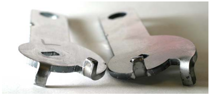
Figure 9: The stops on the flush-handle actuators are opposite. The handles are not interchangeable. The left-side handle is shown on the left above.
